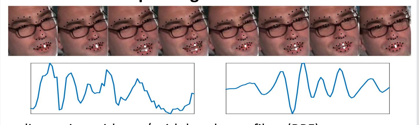
lip motion without / with band-pass filter (BPF) (3.75 – 7.5Hz)
